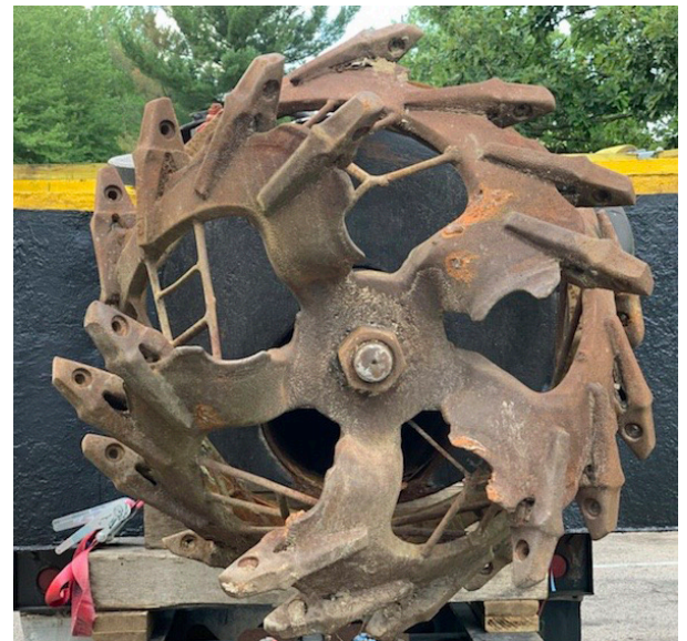
The cutter head hydraulic dredge awaits placement into the Schuylkill River earlier this summer. The cutter head moves through the sediment, which mixes with water to create a slurry that can be pumped into collection barges.
